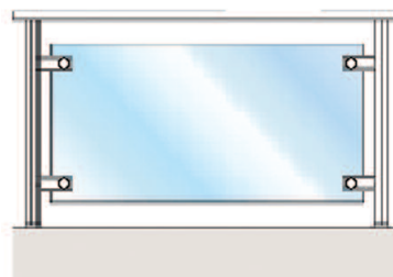
Figure 10 Bolt fixed infill panel
